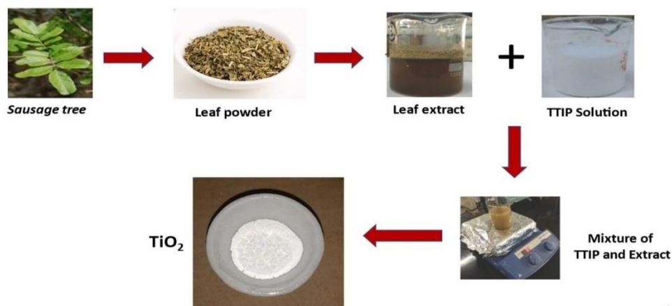
Fig. 2: Diagrammatic representations for Synthesis of TiO 2 NPs.
